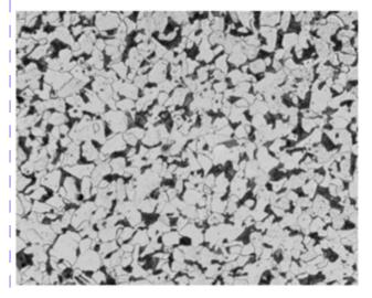
Fine Grained steels are more ductile than coarse grained as Coarse Grained steels have slightly higher tensile and yield strengths than Fine Grained steels. Fine Grain steels are less susceptible to grinding cracks,Less distortion in heat treatment, Higher ductility at the same hardness, Higher impact strength at the same hardness, Higher elastic ratio, Higher % elongation
