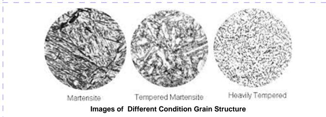
Martensite results from quenching medium- or high-carbon steel. Tempering reduces martensite grain size. Fine-grained martensite are more ductile and tough when compared to coarsegrained ones.
